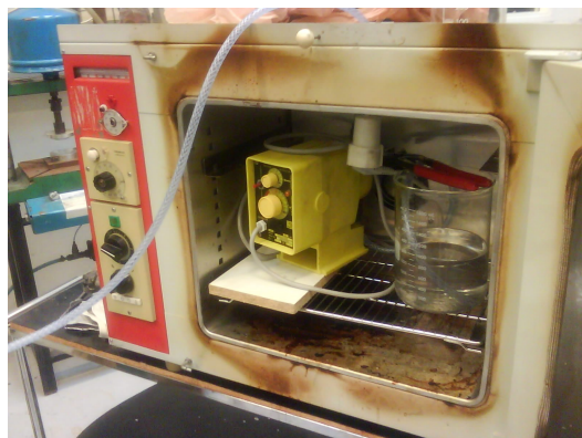
Figure 3. Liquid PCM and pump were held at 40°C in an oven.
