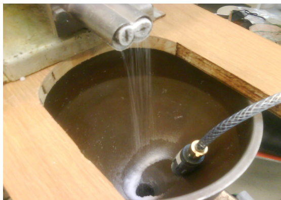
Figure 2. Liquid PCM was fed through a hose down into the hopper.
